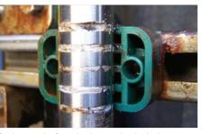
Crevice corrosion formed under a regular plastic clamp
