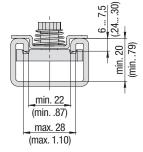
Basic dimensional requirements for channel rails to be used with STAUFF Channel Rail Adaptors, type CRA
