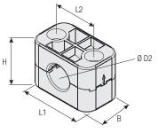
For Use with Compact Hose (Upper Clamp Half rotated by 180°)
